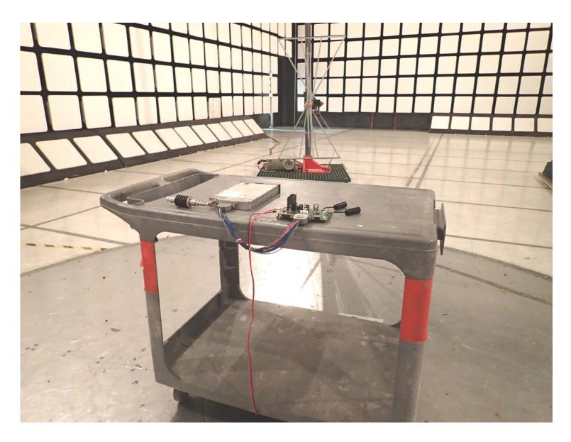
Radiated Transmitter Emission Test at 3m, 30 MHz to 1GHz
