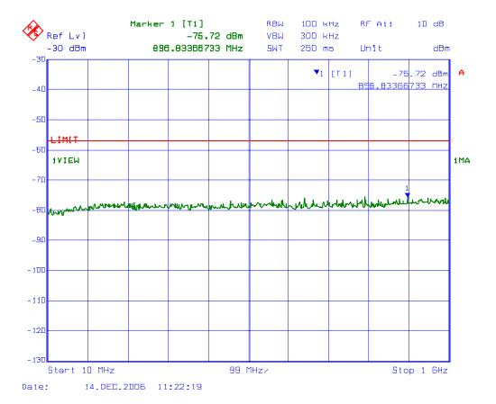
Plot 2: Receiver Antenna Power Conducted Emissions @ Antenna 1
