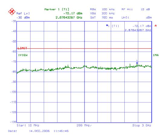
Plot 3: Receiver Antenna Power Conducted Emissions @ Antenna 1
