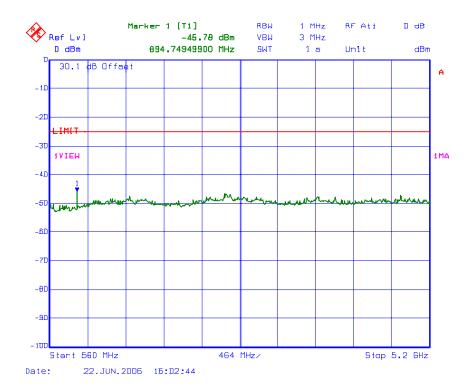
Carrier Frequency (MHz): 450.1 Power (dBm): 30.17 Limit (dBc): 55.17
