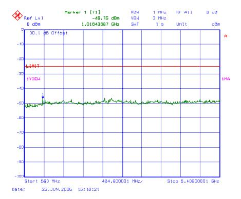
Carrier Frequency (MHz): 511.9 Power (dBm): 29.49 Limit (dBc): 54.49
