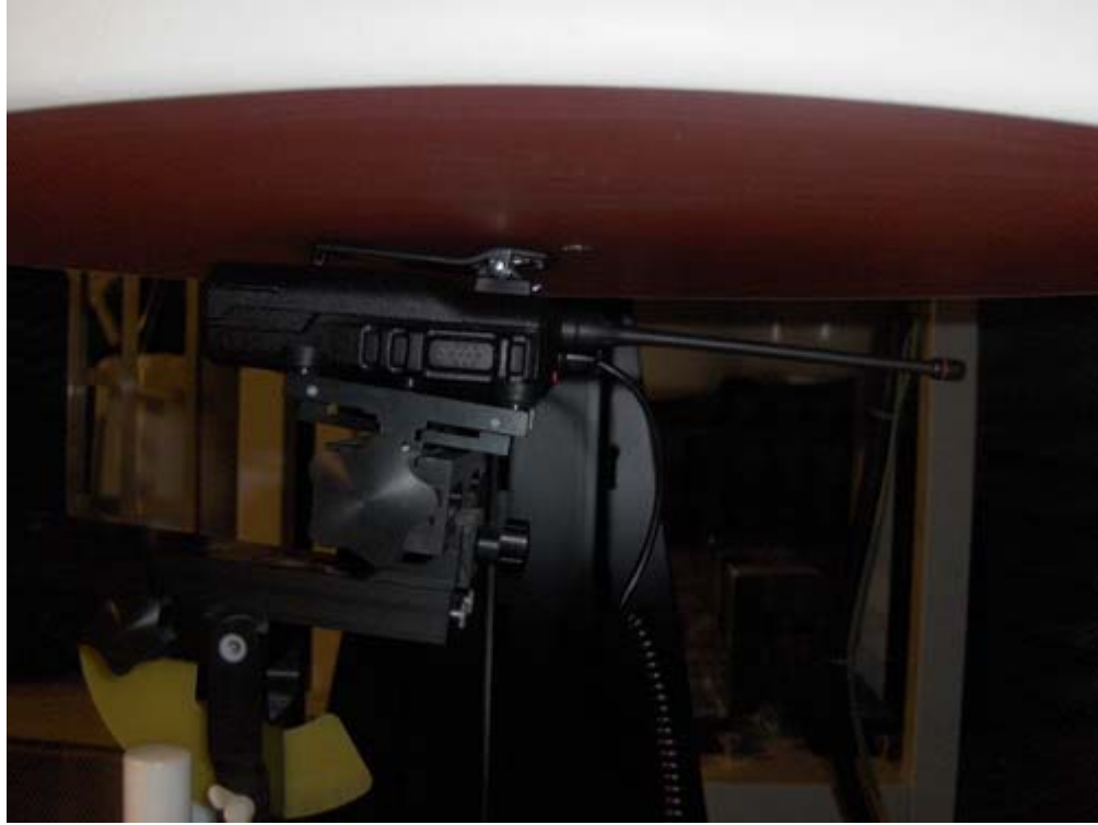
Back side of EUT in parallel to the phantom with the belt-clip (M/N: MB-94) in contact, attached 5 different- type Speaker-microphones separately
