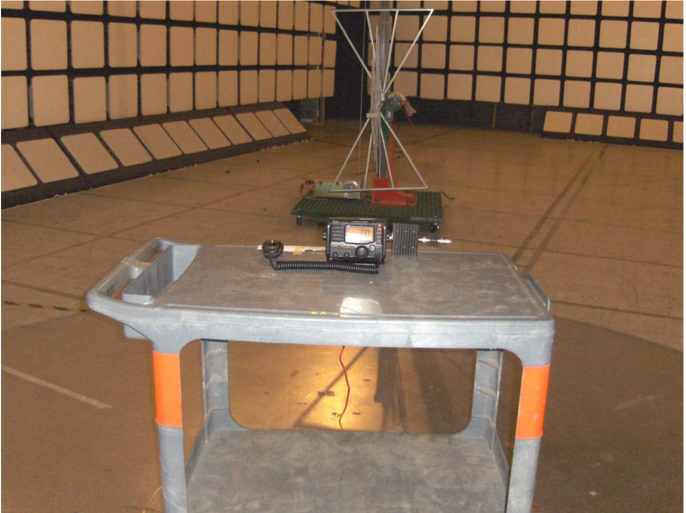
Plot #2: Radiated Emission Test Setup
