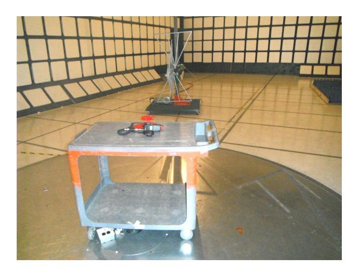
Plot #2: Tx Radiated Emission Test Setup
