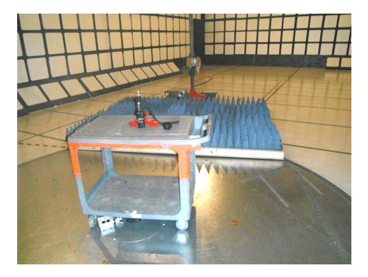
Plot #1: Tx Radiated Emission Test Setup
