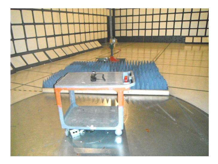
Plot #3: Tx Radiated Emission Test Setup
