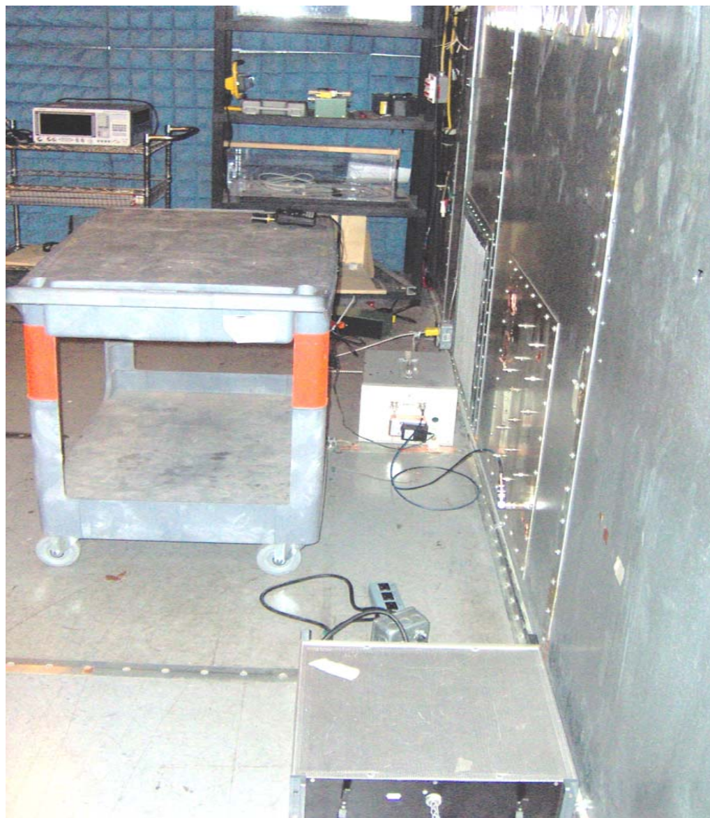
Photo #2: AC Powerline Conducted Emissions
