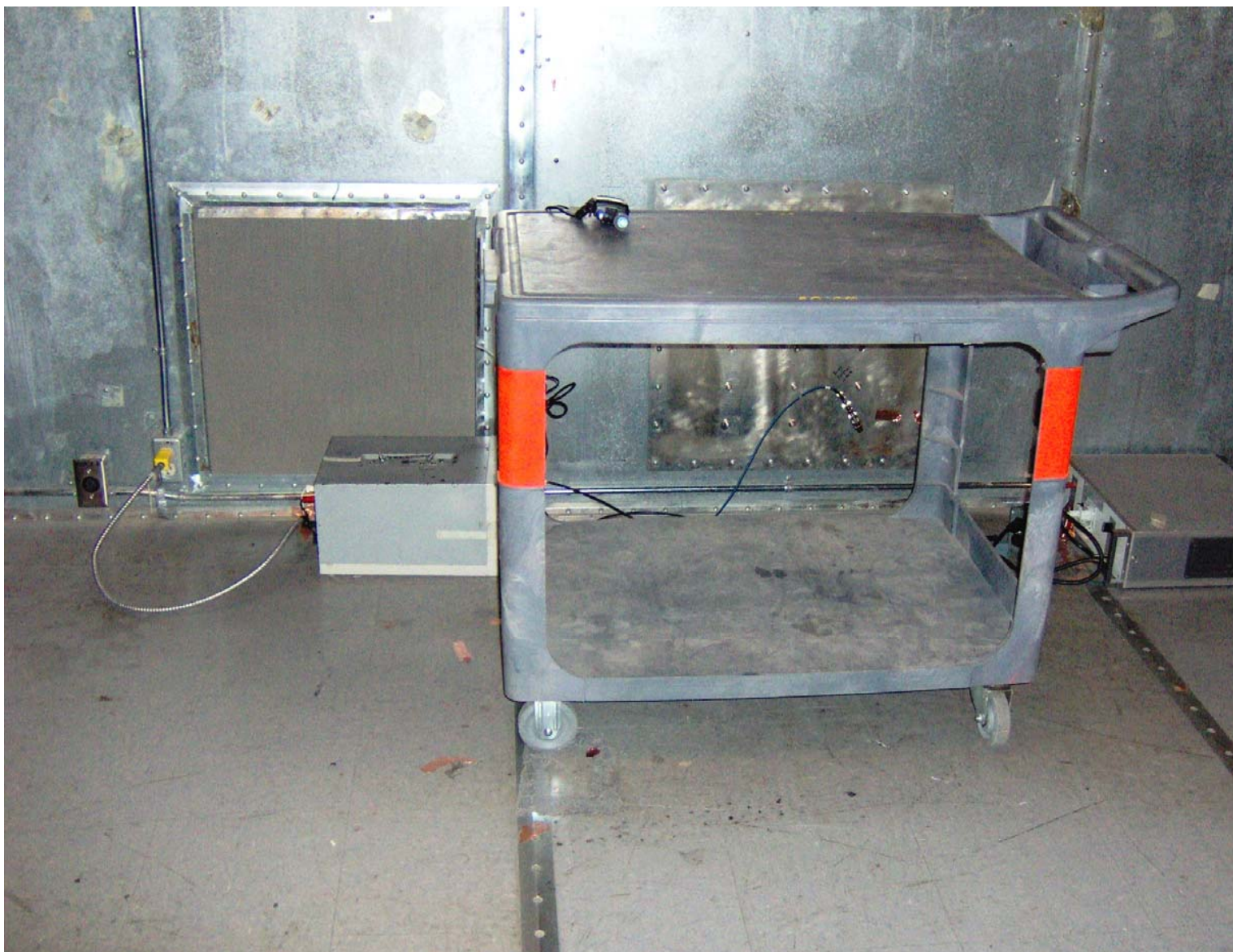
Photo #1: AC Powerline Conducted Emissions
