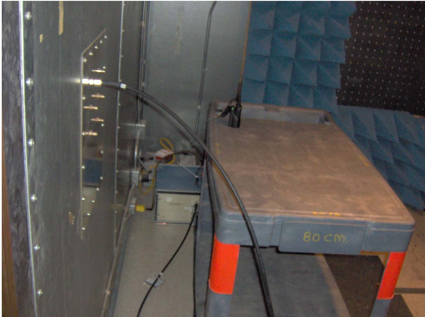
Photo #1: AC Powerline Conducted Emissions
