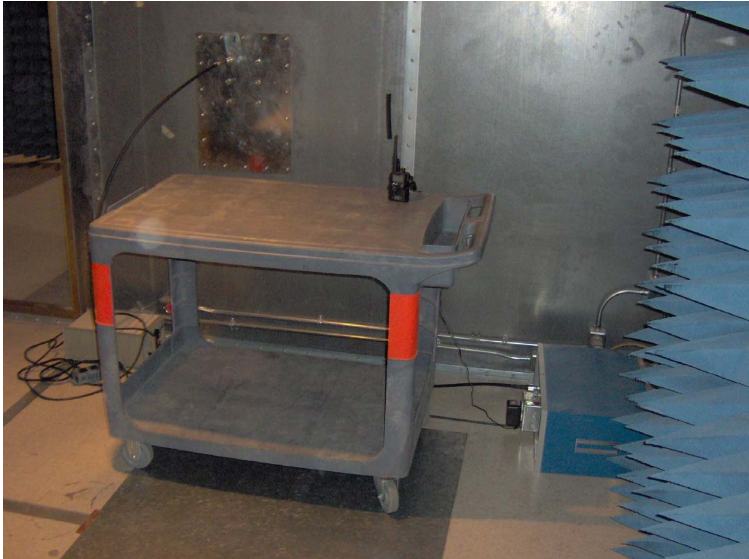
Photo #2: AC Powerline Conducted Emissions
