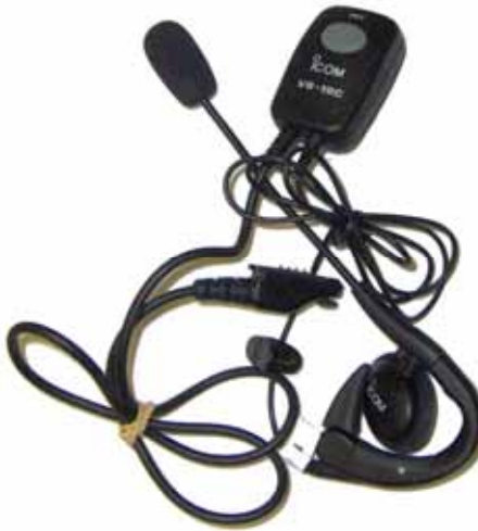
< Headset (M/N: HS-94) + VOX/PTT case (M/N: VS-1SC) >
