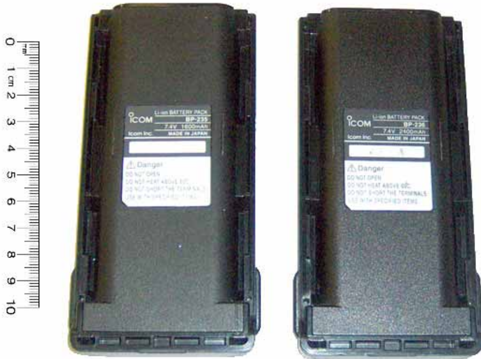
< Li-Ion battery packs (left; M/N:BP-235, 7.4 V, 1600 mAh; right; M/N: BP-236, 7.4 V, 2400 mAh) >
