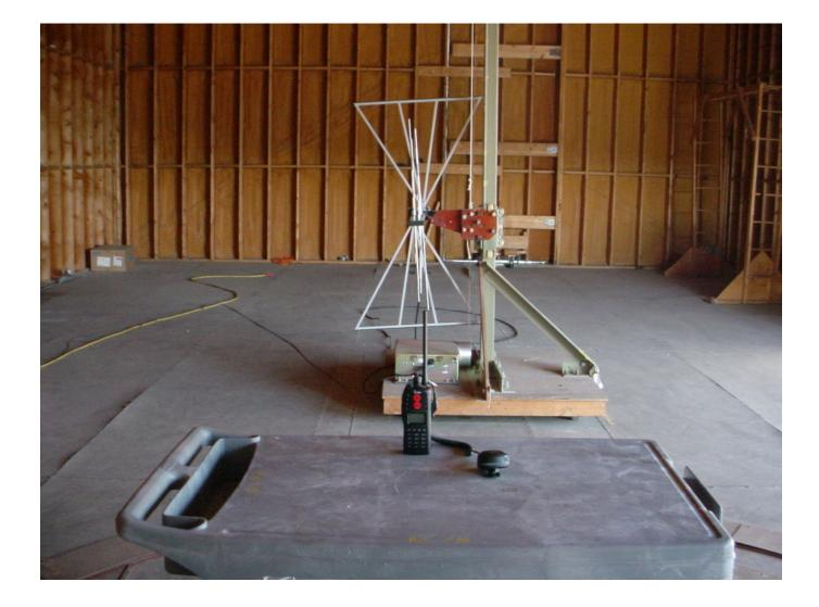
Radiated Emissions Orthogonal Position #1
