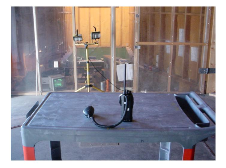
Radiated Emissions Orthogonal Position #1(Rear)
