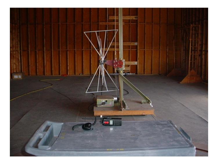
Radiated Emissions Orthogonal Position #3
