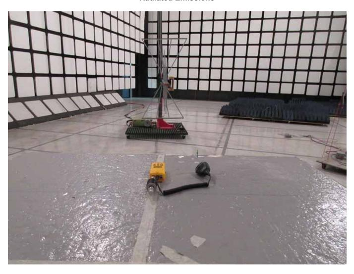
**ANNEX 1 - TEST SETUP PHOTOGRAPHS (Radiated Emissions at 3 Meters Distance)**
