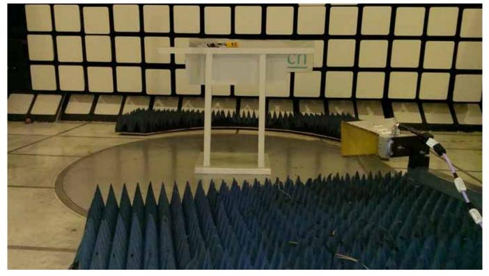
**ANNEX 1 - TEST SETUP PHOTOGRAPHS (Radiated Emissions at 3 Meters Distance)**
