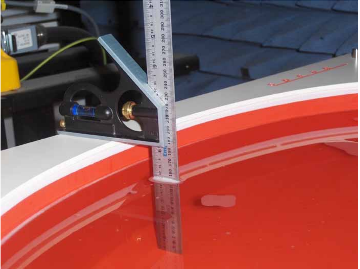
< Phantom filled with body tissue liquid: liquid level = 150mm \pm 5mm >
