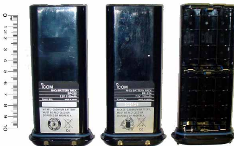
< Ni-Cd battery packs (left; M/N:BP-225, 7.2 V, 1100 mAh; middle; M/N: BP-224, 7.2V, 750 mAh) and battery case (right; M/N: BP-223, 6 × AA(R6) alkaline cells) >
