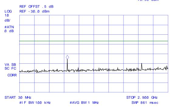
Plot # 4: **Receiver Antenna Port Power Conducted Emissions Receive Test Frequency: 1000 MHz**
