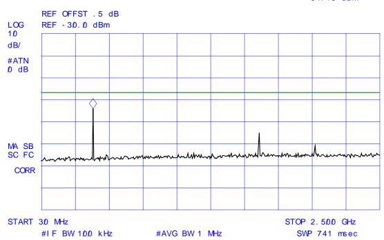
Plot # 3: Receiver Antenna Port Power Conducted Emissions
