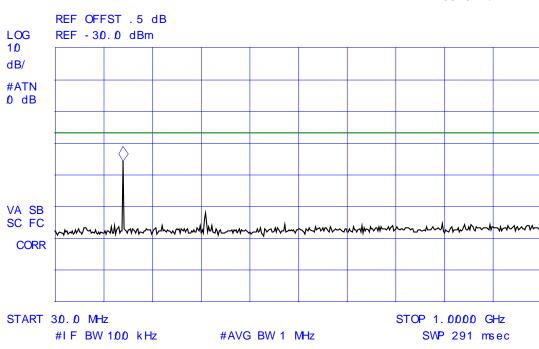
Plot # 2: Receiver Antenna Port Power Conducted Emissions
