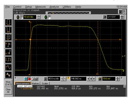
Plot 5.6.4.5: 70% Amplitude Pulse Width, PL3 (2 nm Range)
