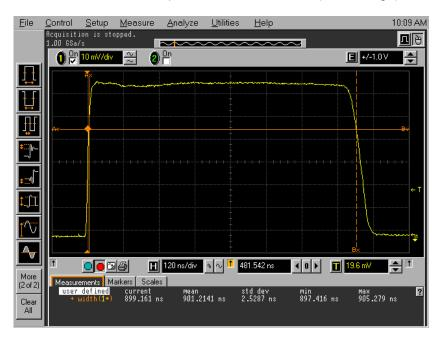
Plot 5.6.4.9: 70% Amplitude Pulse Width, PL5 (8 nm Range)
