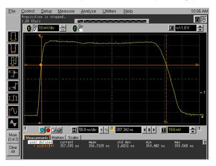
Plot 5.6.4.7: 70% Amplitude Pulse Width, PL4 (4 nm Range)
