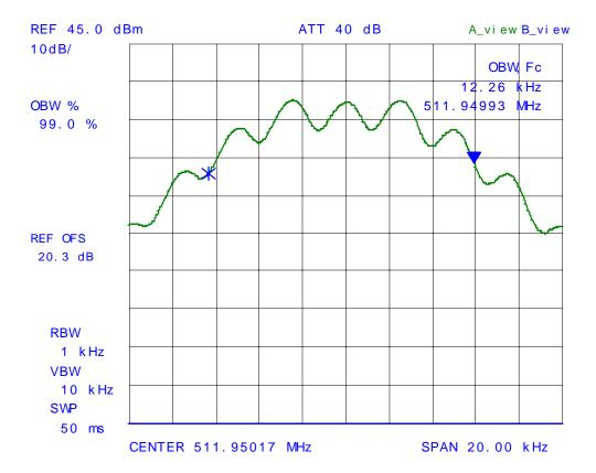
Plot # 7: 99% Occupied Bandwidth, Carrier Frequency: 450.05 MHz Channel Spacing: 12.5 kHz, Power: 4 W
