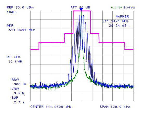
Plot # 19: Emission Mask B, Carrier Frequency: 450.05 MHz
