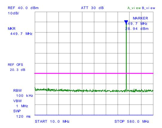
Plot # 40: Spurious Emissions at Antenna Terminal, Carrier Frequency: 450.05 MHz
