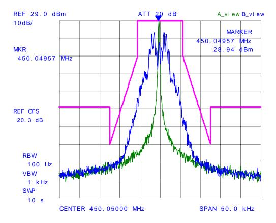
Plot # 35: Emission Mask D, Carrier Frequency: 485.05 MHz
