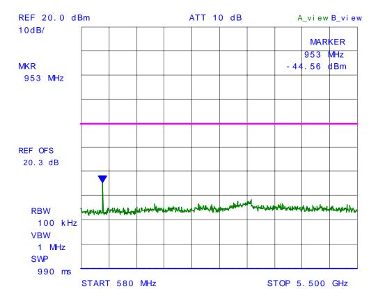
Plot # 43: Spurious Emissions at Antenna Terminal, Carrier Frequency: 485.05 MHz
