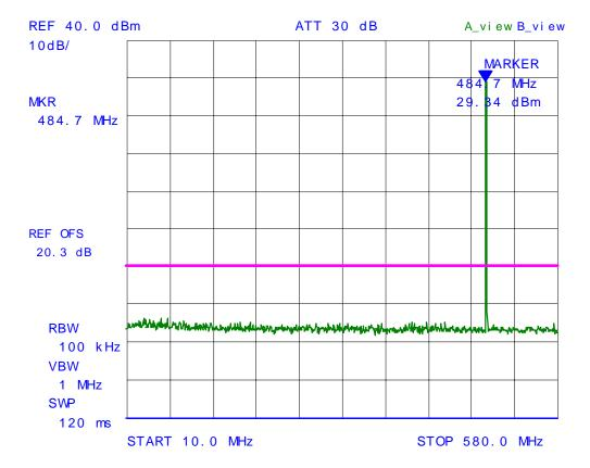
Plot # 44: Spurious Emissions at Antenna Terminal, Carrier Frequency: 485.05 MHz
