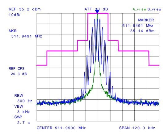
Plot # 16: Emission Mask B, Carrier Frequency: 450.05 MHz
