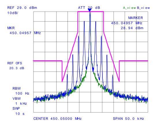
Plot # 29: Emission Mask D, Carrier Frequency: 485.05 MHz
