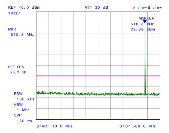
Plot # 48: Spurious Emissions at Antenna Terminal, Carrier Frequency: 511.95 MHz
