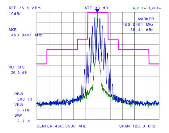
Plot # 14: Emission Mask B, Carrier Frequency: 485.05 MHz
