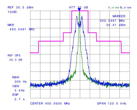
Plot # 20: Emission Mask B, Carrier Frequency: 485.05 MHz
