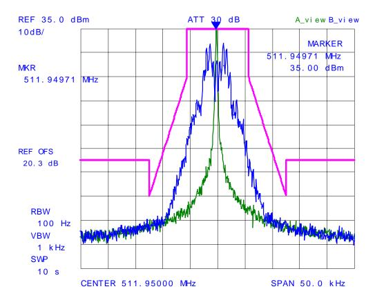
Plot # 34: Emission Mask D, Carrier Frequency: 450.05 MHz
