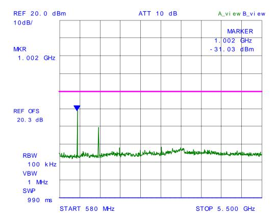
Plot # 47: Spurious Emissions at Antenna Terminal, Carrier Frequency: 511.95 MHz
