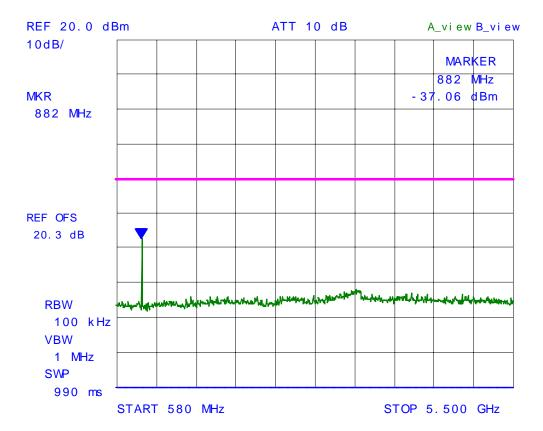
Plot # 39: Spurious Emissions at Antenna Terminal, Carrier Frequency: 450.05 MHz
