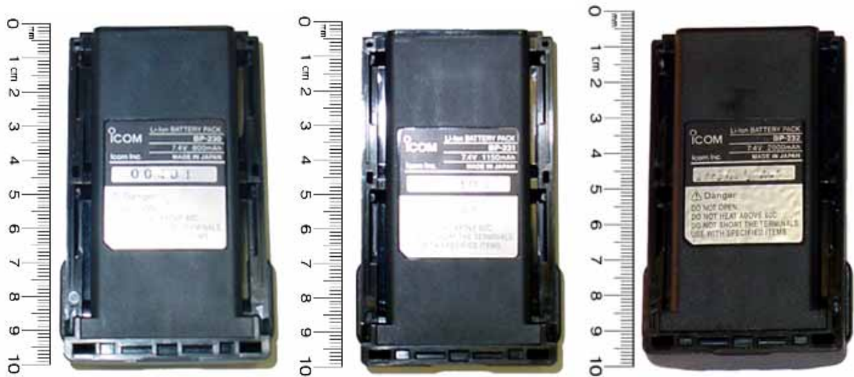
< Li-Ion battery packs (left; M/N:BP-230, 7.4 V, 800 mAh; middle; M/N: BP-231, 7.4V, 1150 mAh; right; M/N: BP-232, 7.4 V, 2000 mAh) >
