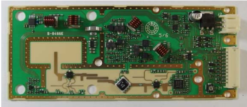
RECEIVER Unit A side
