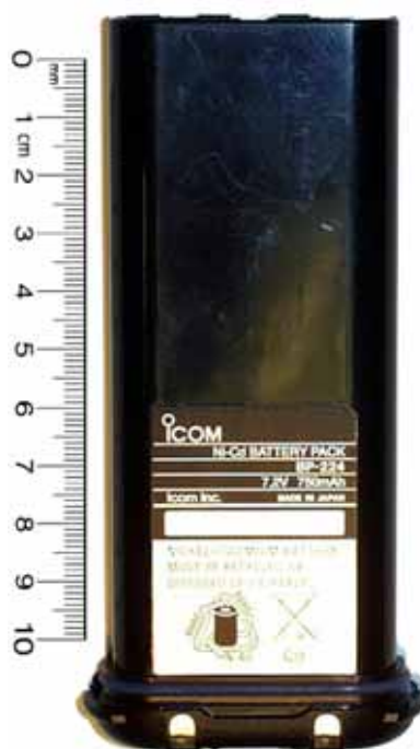
< Rechargeable Ni-CD battery pack (M/N:BP-224, 7.2 V, 750 mAh) >
