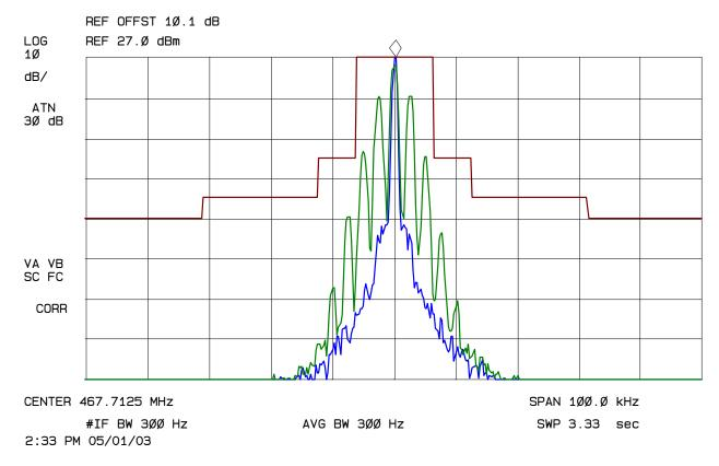
Plot 12: **Emission Limitation** Carrier Frequency: 467.7125 MHz (CH 14) Modulation: FM with 2.5 kHz sine wave Voice Scrambler Function: ON CTCSS Code: OFF
