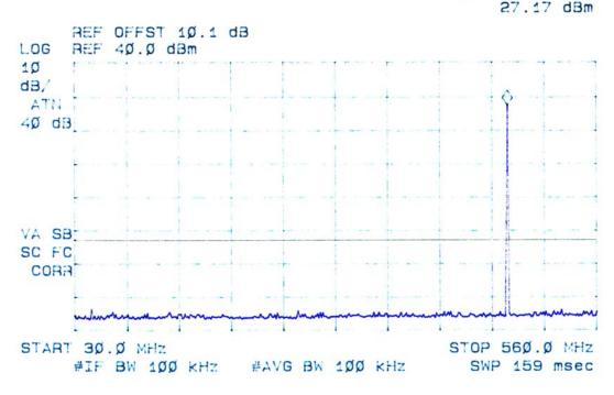
Plot 19: Spurious Emissions at Antenna Terminals Carrier Frequency: 467.7125 MHz (CH 14) Modulation: FM with 2.5 kHz sine wave
