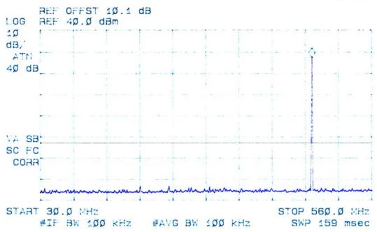
Plot 16: Spurious Emissions at Antenna Terminals Carrier Frequency: 462.5625 MHz (CH 01) Modulation: FM with 2.5 kHz sine wave
