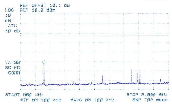
Plot 17: Spurious Emissions at Antenna Terminals Carrier Frequency: 462.5625 MHz (CH 01) Modulation: FM with 2.5 kHz sine wave
