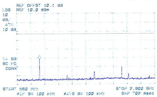
Plot 20: Spurious Emissions at Antenna Terminals Carrier Frequency: 467.7125 MHz (CH 14) Modulation: FM with 2.5 kHz sine wave
