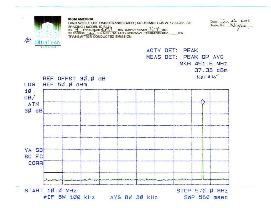
MOBILE UHF TRANSCEIVER, Model IC-F221
