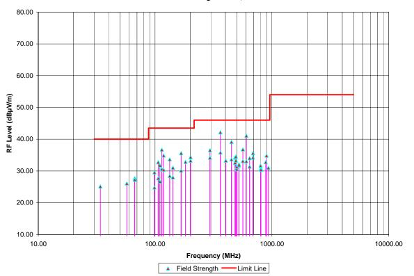
Radiated Emissions Measurements @ 3m OFTS ICOM Scanning Receiver, Model: 7800
