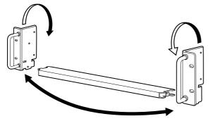
3 Attach the handles to the bar, then tighten the screws.
