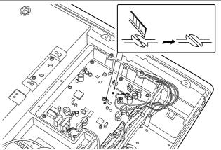
**NOTE:** Be sure to re-solder above disconnected points, otherwise no TX modulation or AF output is available when you remove the scrambler unit.
