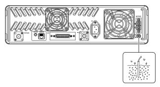
⚠ **WARNING: NEVER** connect the [GND] terminal to a gas or electric pipe, since the connection could cause an explosion or electric shock.
