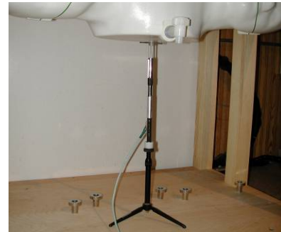
Figure 12-2 System Verification Setup Photo
