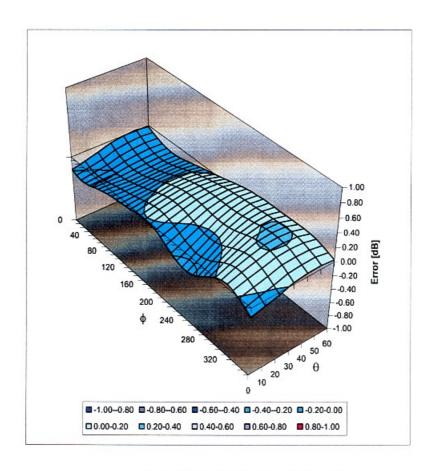
Spherical Isotropy Error < ± 0.4 dB
