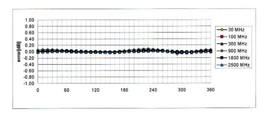
Axial Isotropy Error < ± 0.2 dB
