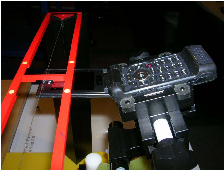
Figure 17-1 Ear Reference Point HAC Phantom Alignment
