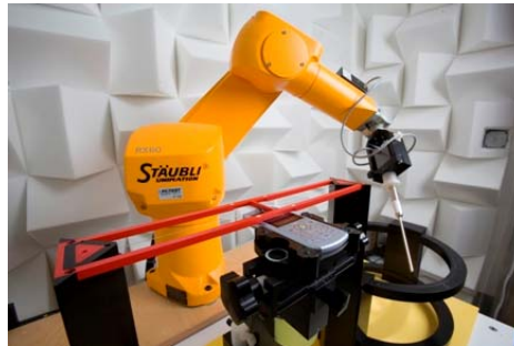
Figure 5-5 SPEAG Robotic System
