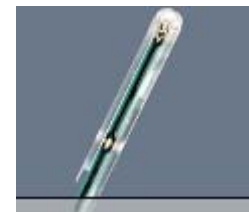
Figure 5-2 H-Field Free-space Probe
