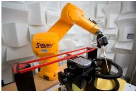
Figure 5-5 SPEAG Robotic System
