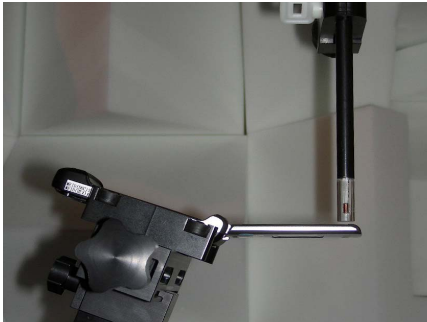
Figure 13-2 Test Setup for Wireless Device
