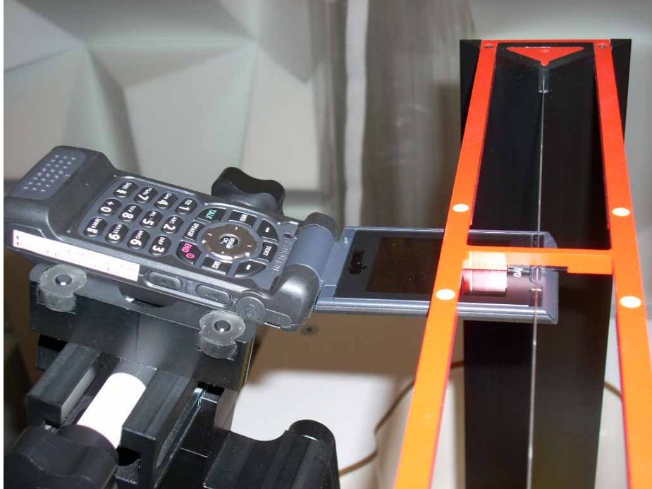
Figure 17-1 Ear Reference Point HAC Phantom Alignment
