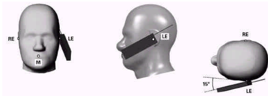
Figure 9.3 Front, Side and Top View of Ear/15° Tilt Position
