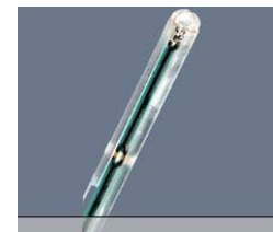
Figure 5-2 H-Field Free-space Probe
