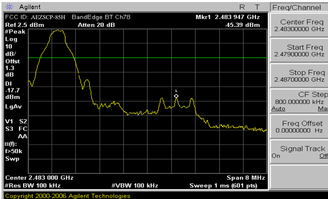
Plot 6-5. Band Edge Plot (Bluetooth – Ch. 78)
