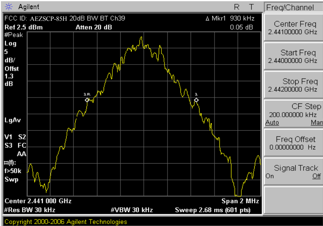
Plot 6-2. 20dB Bandwidth Plot (Bluetooth – Ch. 39)
