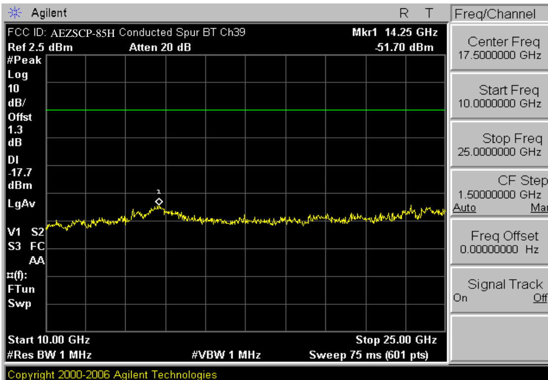
Plot 6-13. Conducted Spurious Plot (Bluetooth – Ch. 39)
