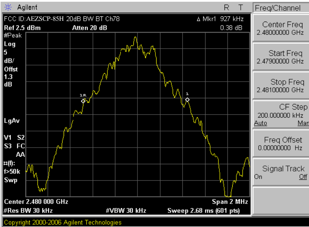
Plot 6-3. 20dB Bandwidth Plot (Bluetooth – Ch. 78)
