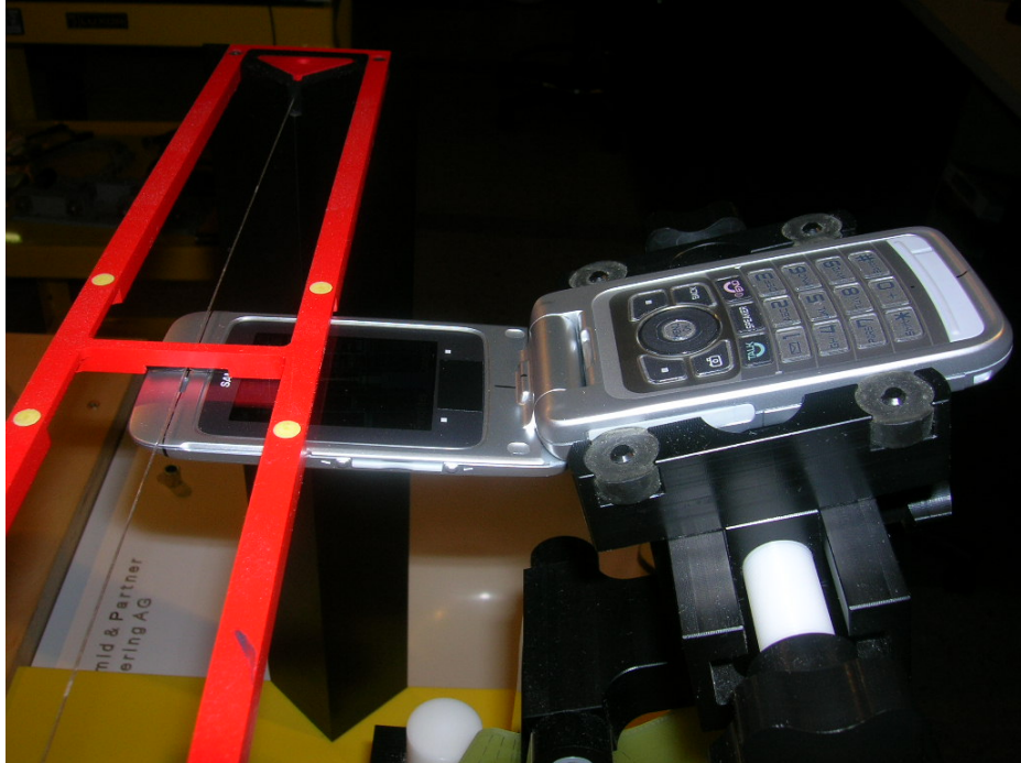
Figure 17-1 Ear Reference Point HAC Phantom Alignment
