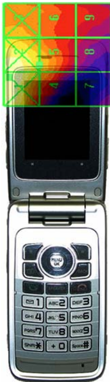
Figure 17-4 E-Field WD Scan overlay
