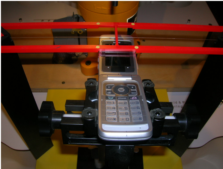
Figure 17-2 HAC Phantom Plane Alignment
