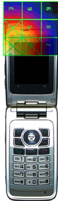
Figure 17-5 H-Field WD Scan overlay
