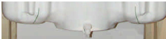
Figure 7.2 SAM Twin Phantom shell
