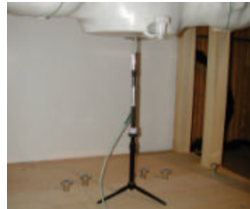
Figure 12.1 Dipole Validation Test Setup
