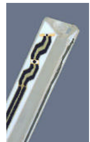
Figure 3.2 Probe Thick-Film Technique
