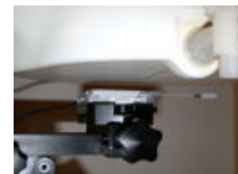
Figure 14.14 Body SAR Test Setup -- w/o Holster --
