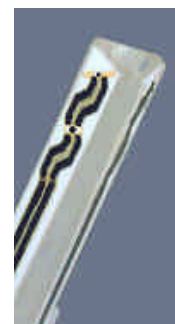
Figure 3.2 Probe Thick-Film Technique
