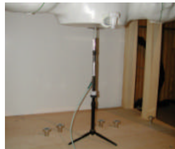
Figure 12.1 Dipole Validation Test Setup
