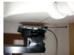
Figure 14.15 Body SAR Test Setup -- w/o Belt-clip --
