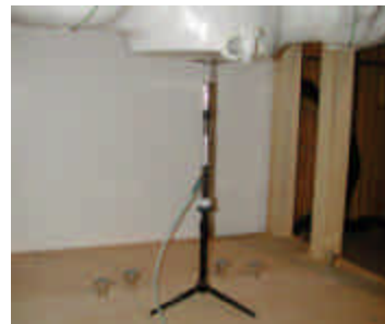
Figure 12.1 Dipole Validation Test Setup
