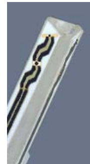
Figure 4-2 Probe Thick Film Technique
