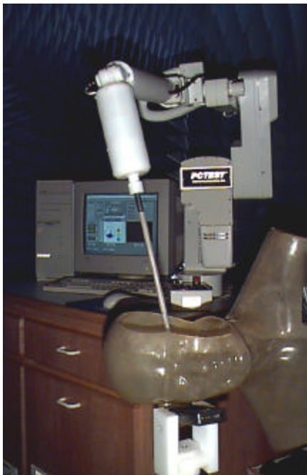
Figure 5. Photograph of the Probe and the Phantom
