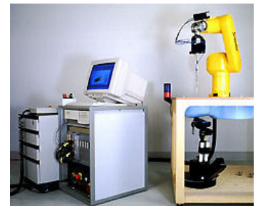
Fig. 1 SAR Test Setup
