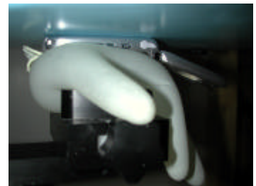
Figure 21. Hand SAR Test Setup
