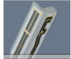
Figure 4 E-field Free-space Probe
