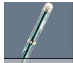
Figure 5 H-Field Free-space Probe
