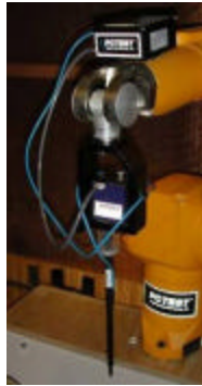
Figure 9 SPEAG Robotic System
