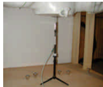
Figure 12.1 Dipole Validation Test Setup
