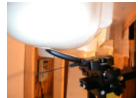
Figure 14.10 Right Head SAR Test Setup -- Ear / Tilt Position --
