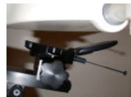
Figure 14.18 CDMA Face SAR Test Setup -- Flip Open Position --
