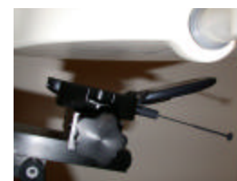
Figure 14.16 AMPS Face SAR Test Setup -- Flip Open Position --
