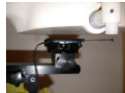
Figure 14.14 Body SAR Test Setup -- w/o Holster --
