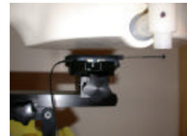
Figure 14.15 Body SAR Test Setup -- w/o Holster --
