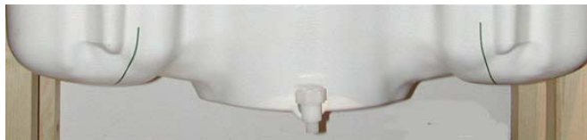
Figure 7.2 SAM Twin Phantom shell
