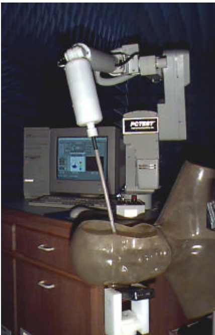
Figure 5. Photograph of the Probe and the Phantom
